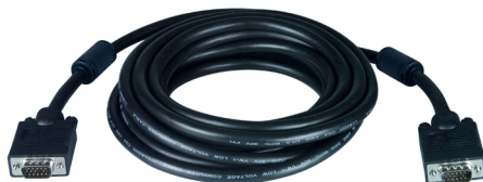
Male 15HD Male 15HD VEXT-PLNM-25/50/75/100-MM Plenum VGA male to male cable 0.30" diameter 25 to 100 feet
