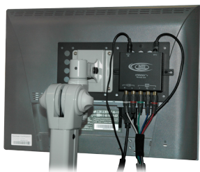
Remote unit mounted to the back of a flat panel monitor using ST-C5MK-VESA mounting kit
